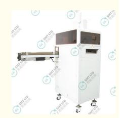
**GS-JBT2101(Monorail)**A DIMM feeder is a component supply device that neatly arranges multiple stacked disk DIMM slots and sends them out one by one at a specified time to supply the insertion machine.
