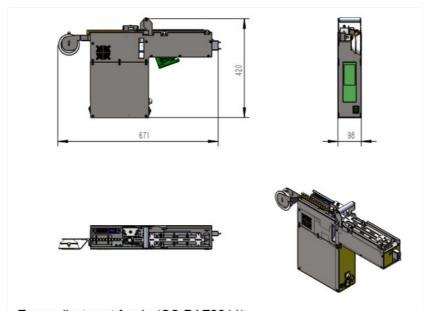
Tape adjustment feeder(GS-RAZ2211) Schematic diagram of appearance and dimensions (Unit:mm)
